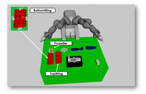
Fig. 1. Motivating example in assembly domain showing cases that need the planner to use the failure ontology to interpret query and action results. Description of reachability and collision problems. The sequence of assemble the Battat toy can be found in https://sir.upc.es/projects/ontologies/
