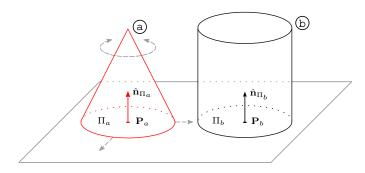
Fig. 1. The mobile object a is constrained with respect to the fixed object b according to the *plane-plane* coincidence constraint  $\Pi_a = \Pi_b$ . The available DOF of a (one rotation, two translations) are shown as dashed lines.
