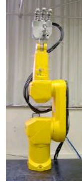
Fig. 2. CAD models of the dexterous hand MA-I and the Stäubli RX90 robot and the physical hand-arm ensemble.
