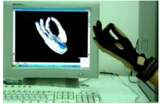
Fig. 2. Human hand with the sensorized glove connected to the mechanical hand simulator used in the data acquisition procedure.
