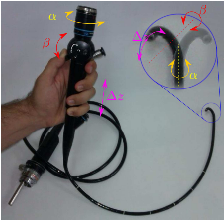
Fig. 2. Degrees of freedom of a bronchoscope: Advance \Delta z , twist \alpha and bending \beta .
