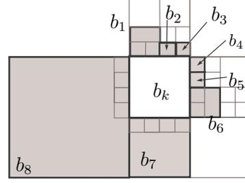
Fig. 2. Neighbor cells of different size used to compute the harmonic function at  $b_k$ . Cells  $b_2$ ,  $b_3$ ,  $b_4$  and  $b_5$  are  $M$ -cells.
