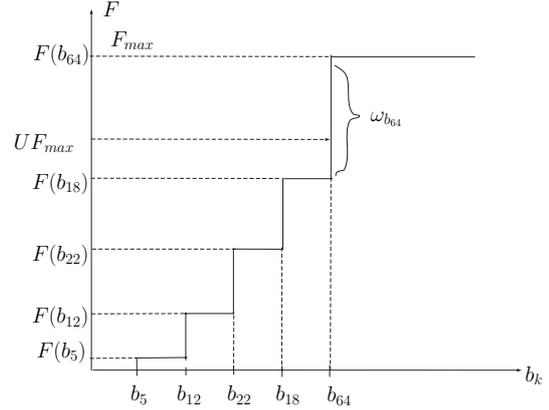
Fig. 5. Random sampling using cumulative function  $F(b_k)$ . A randomly chosen value  $U \in [0, 1]$  determined that cell  $b_{64}$  be chosen.
