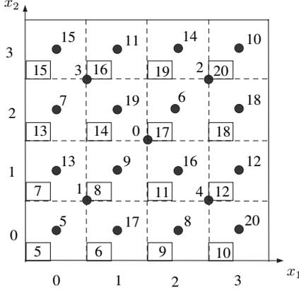
Fig. 3. Sampled configurations of a 2D  $\mathcal{C}$ -space located at the center of the sampled cells. The configuration labels indicate the index in the generation sequence. Boxed numbers are the codes of the 2-cells.
