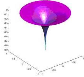
Fig. 2. The landscape of the harmonic function shows the flat region problem encountered far from the goal configuration  $\mathbf{r}_d$  where a delta function is located.
