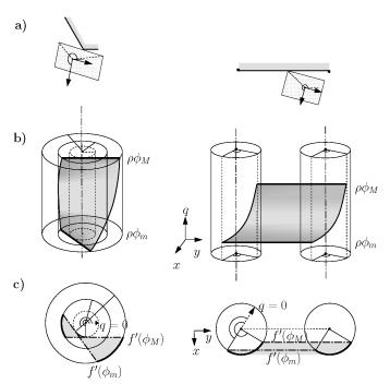
**Figure 1.** Type-A and a type-B basic contacts in (a) physical space; (b) C-space and (c) C'-space.
