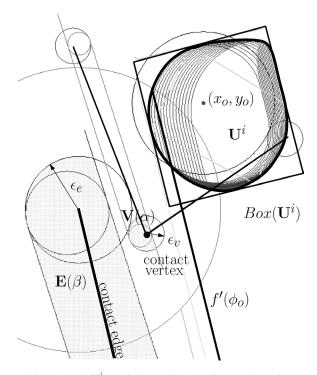
**Figure 6.** Contact position domain  $U^i$  and its bounding box for an orientation  $\phi_0 > \phi_M$ .
