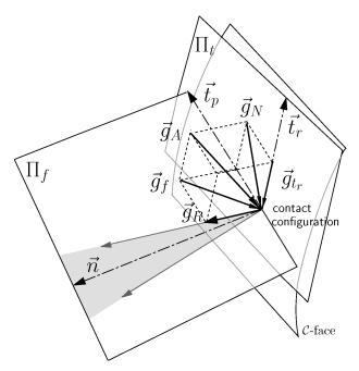
**Figure 2.** Force decomposition in C-space.
