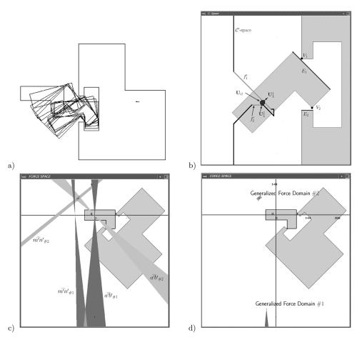
**Figure 14.** (a) Solution path in  $C_{\text{free}}$ ; (b) contact position domains used for the compatibility analysis; (c) dual space force analysis and (d) generalized force domains used for the distinguishability analysis.
