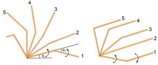
Fig. 3. Left: Motion of the 2 DOF planar robot along the first PMD that defines a positive coupling between the two joint angles  $\theta_1$  and  $\theta_2$ , i.e. both joints move in the positive (counterclockwise) sense. Right: Motion along the second PMD that defines a negative coupling, i.e.  $\theta_1$  moves counterclockwise while  $\theta_2$  moves clockwise.
