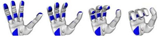
Fig. 2. Configurations of the SAH hand when it is moved along the first PMD (i.e. with only one DOF). Reproduced from [21].
