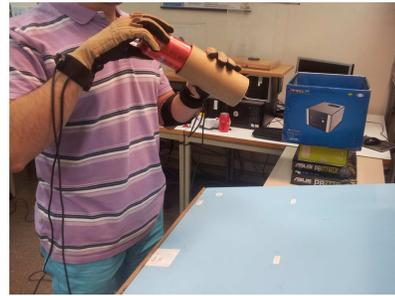
Fig. 2. Human operator performing a task with both hands while wearing the measurement equipment.
