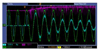
waveform (230Vrms 50Hz), in light blue the AC mains current and in magenta the DC output voltage. Note how the input current is sinusoidally shaped when the algorithm starts and how the DC output voltage is increased, as required.
